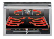
Balanced heat distribution is essential when baking, roasting, and dehydrating food. The American Range convection oven technology features a convection motor and louvered side panels to enhance uniform heat distribution throughout the large oven cavity.
