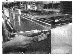
2. Slide the rear island trim between the back panel and existing island back. The holes on the trim will align with the holes of the 6 screws you removed.
